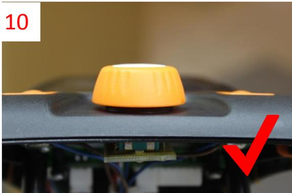
10/ Carefully refit the control knob fully down. Do not push down at an angle as this could damage the speed controller shaft.
