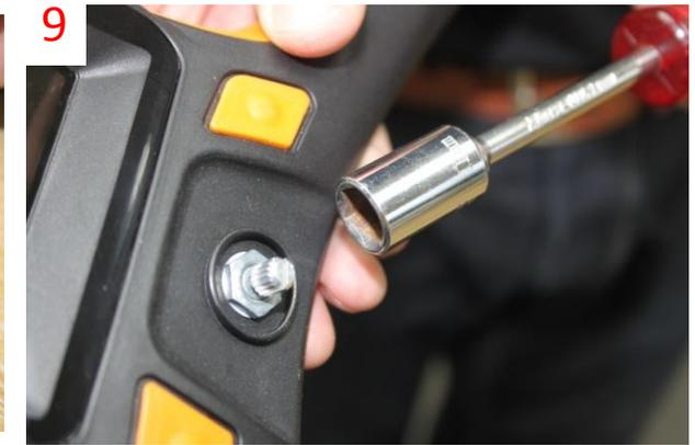
**9/** Refit the speed controller locking nut and washer. Take care to ensure it is laying flat against the inside of the handle housing. Do not to over tighten.
