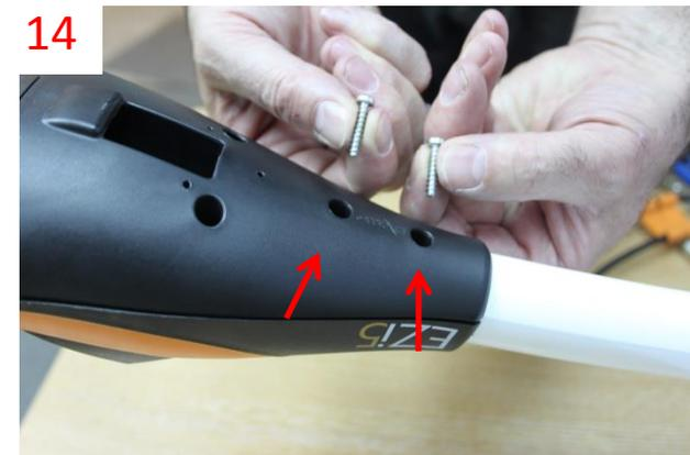
14/ Refit the rear cover moulding. Ensure the two long screws go in the positions shown. Take care not over tighten the screws and that no wires are trapped between the two halves..
