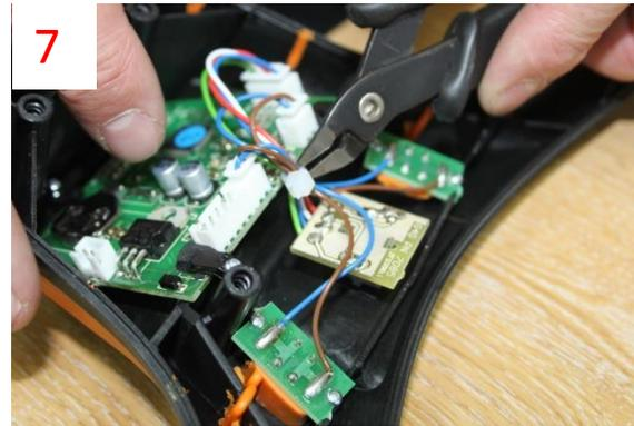
**7/** Carefully cut and discard the cable tie. Take care not to damage any wires. Unplug the encoder lead from the LCD PCB.
