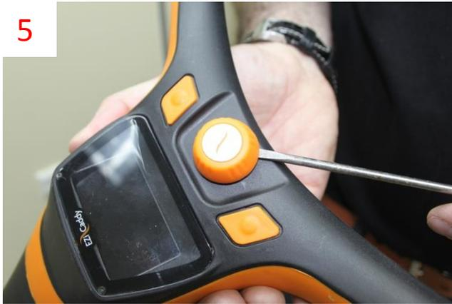
**5/** Using the flat blade screwdriver carefully remove the control knob. Try to lift evenly all round so as not to damage the speed control shaft.
