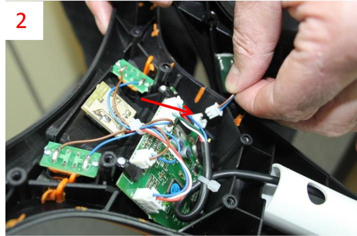
**2/** Carefully disconnect the USB supply and put the handle lower moulding aside.
