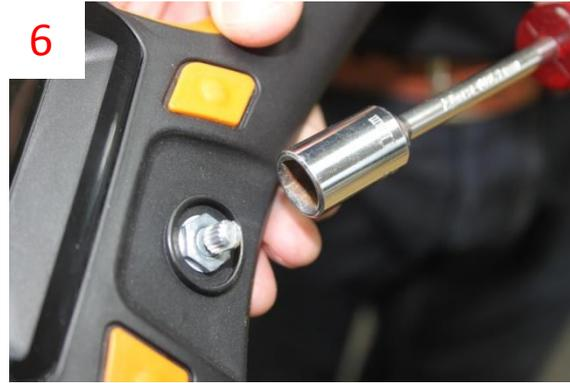
**6/** Remove the speed controller locking nut and washer with the 11mm socket and remove the speed controller from the handle.
