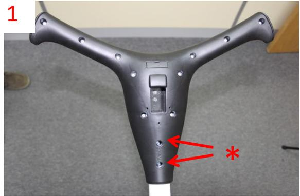
**1/** Unfold the Trolley and position it upside down on the floor to get easy access to the underside of the handle and remove all 12 screws with a PZ2 screwdriver. \*Take note of the position of the two longer screws as indicated \*.
