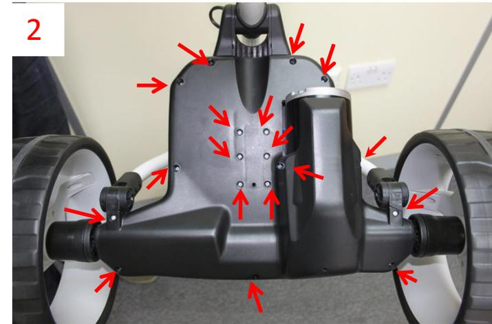
2/ Remove all screws as shown with a Pozidrive No2 Screw driver.
