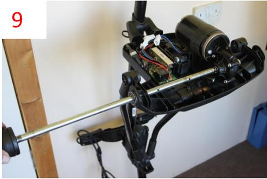
**9/** Slide the axle out to the left and remove.
