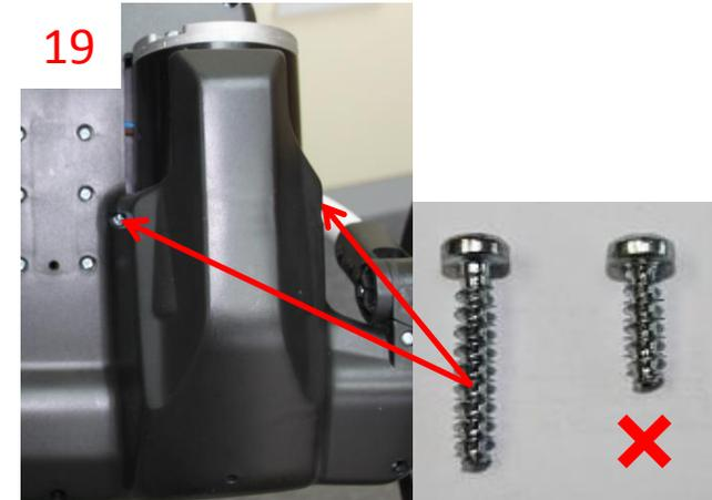
19/ Refit all the case screws. Make sure the two longer case screws are in the positions shown. Take care not over tighten the screws.
