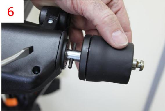
6/ Remove the wheel and clutch from the right hand side.
