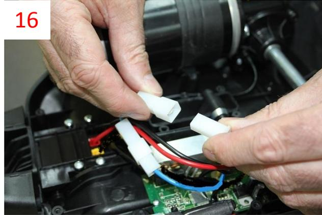
16/ Reconnect the two white connectors that hold the **Brown** and **Blue** wires.
