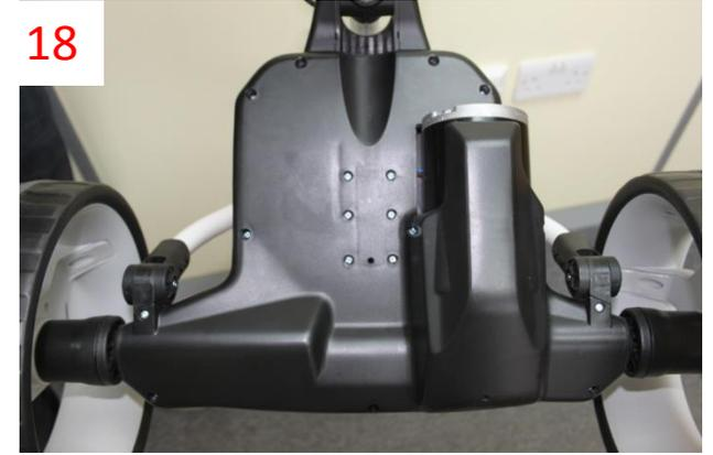
18/ Refit the rear cover ensuring no wires or moving parts are trapped between the cases. Also refit the clutch and wheels.
