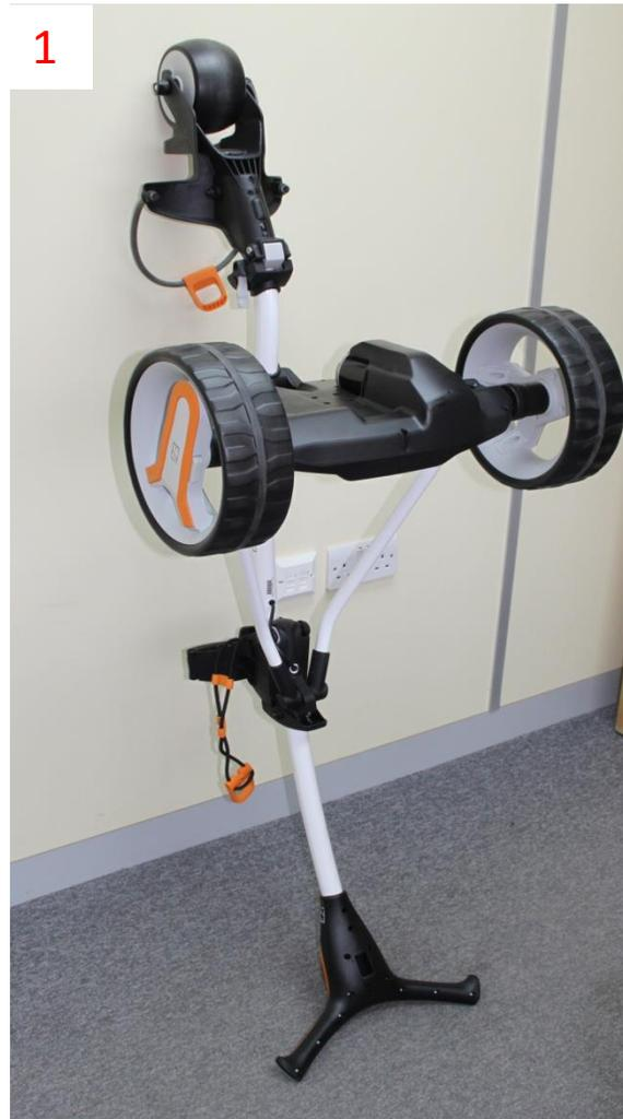
1/ Stand cart against a wall as shown to give easy access to the underneath of the cart.
