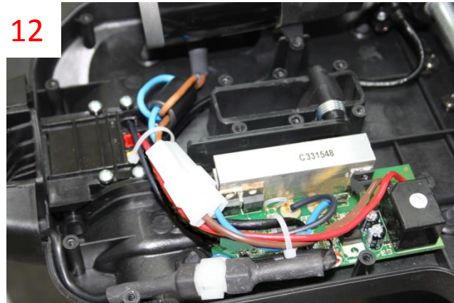
12/ With all wires connected, loosely attached two cable ties around wires in positions shown and trim any excess. Carefully route the wires as shown in the picture.
