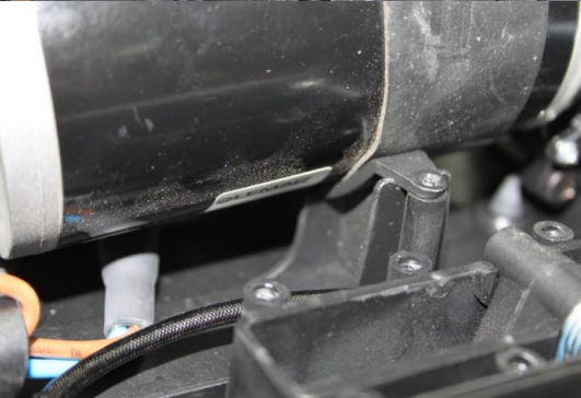
10/ Ensure the motor mount is correctly positioned and the motor is seated correctly.
