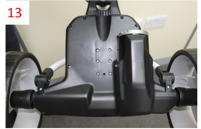
13/ Refit the rear cover ensuring no wires or moving parts are trapped between the cases.
